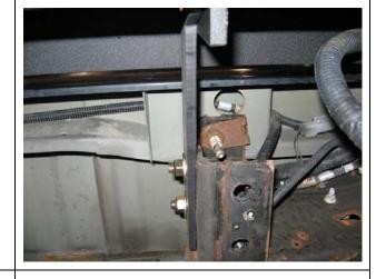
10. Remove the factory plate lamp connector from the end of the wire harness. Connect the wire terminals to the end of the factory wire loom.
