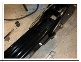
27.1 Connect short hoses (25" long) to the corresponding color hoses from the elbow. Route the hoses through the ram so the exit out the end, one on each side of the cylinder pin mounting tube on the ram.
