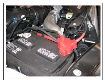
19.1 Install a 12 Volt deep cycle marine battery into the battery box on the Minute Man frame. It is recommended to have a battery that has a minimum of 500 Cold Cranking amps (CCA rating).
