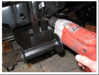
6. Place the counterweight back in position (if moved) and bolt in place using the included bolts and nuts. If the included hardware is not of sufficient, replace with Grade 8 or higher quality fasteners. Always install the rear most bolt first so that it is accessable inside the frame.
