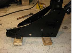
23. The boom should be able to rest in the cradle as the boot touches the ground. The elbow has multiple mounting holes for the boot. Find the combination that works best for the truck.
