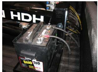
19.2 Connect the 2/0 cable from the grounding screw on the pump manifold to the negative terminal on the auxiliary battery.
