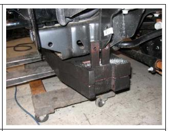
5. If possible drill the holes in the frame with the counterweight in position. If this is not possible, mark the hole locations with spray paint of a transfer punch.
