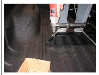
7. Place the rear mounting bracket under the holes drilled through the bed. The upper leg of the bracket must be flush with the truck bed and the lower leg must be flat against the truck frame (shown in the illustration top, right on the following page). For Ford trucks, remove the rear overload spring stop from the truck frame and follow the next three steps.
