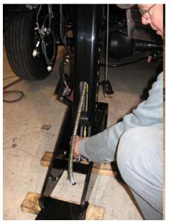
25. Remove the in/out cylinder from the ram and extension by first removing access plug. Then pull out the cylinder pin and remove the cylinder body from the extension. There is a ½" punch access hole opposite the threaded plug hole.
