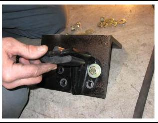
7.3 (Ford Trucks) Position the bracket assembly as shown at the right. Note upper leg of the bracket extends to the outside of the truck frame. Go on to step nine.
