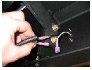
12. Replace the wire loom back around the factory wiring and cover the loom and connectors with electrical tape.
