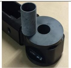
To identify a problem a customer can extend his/her lift out to a ready to tow position with the in/out cylinder fully extended and if a gap in between the head plates and the inner extension (ram) plates exist; the center bolt may need to be tightened or the thrust washer will need to be replaced due to wear.
